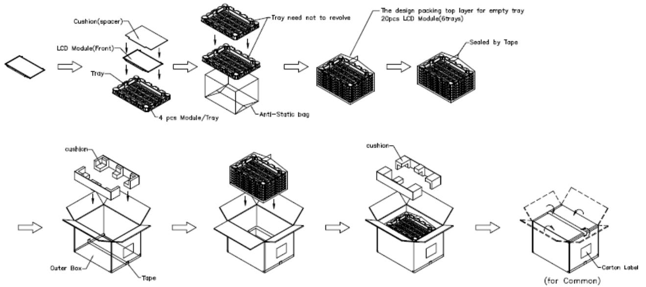
**Figure. 7-1 Packing method**
