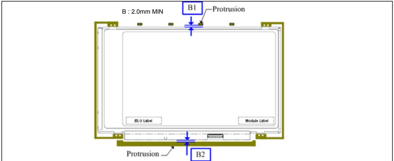
**Definition** Gap between panel & protrusions is needed to prevent shock test failure. Because protrusions with small gap may hit panel during the test. Issue such as cell crack, abnormal display may occur.
