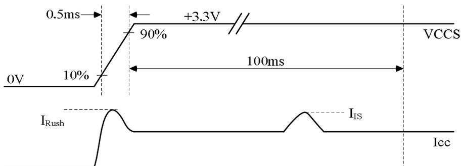
Note (3) The specified power supply current is under the conditions at  $V_{CCS} = 3.3\text{ V}$ ,  $T_a = 25 \pm 2\text{ }^\circ\text{C}$ , DC Current and  $f_v = 60\text{ Hz}$ , whereas a specified power dissipation check pattern is displayed
