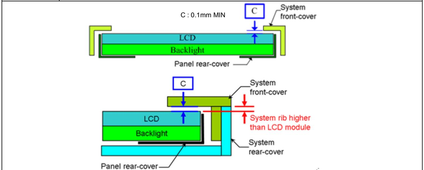
**Definition** Gap between system front-cover & panel surface is needed to prevent pooling or glass broken. Zero gap or interference such as burr and warpage from mold frame may cause pooling issue near system font-cover opening edge. This phenomenon is obvious during swing test, hinge test, knock test, or during pooling inspection procedure. To remain sufficient gap, design with system rib higher than maximum panel thickness is recommended.
