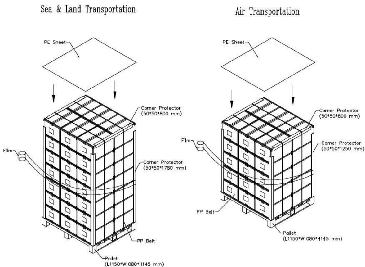
Figure. 7-3 Packing method
