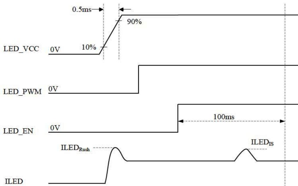
Note (2) If PWM control frequency is applied in the range less than 1KHz, the “waterfall” phenomenon on the screen may be found. To avoid the issue, it’s a suggestion that PWM control frequency should follow the criterion as below.
