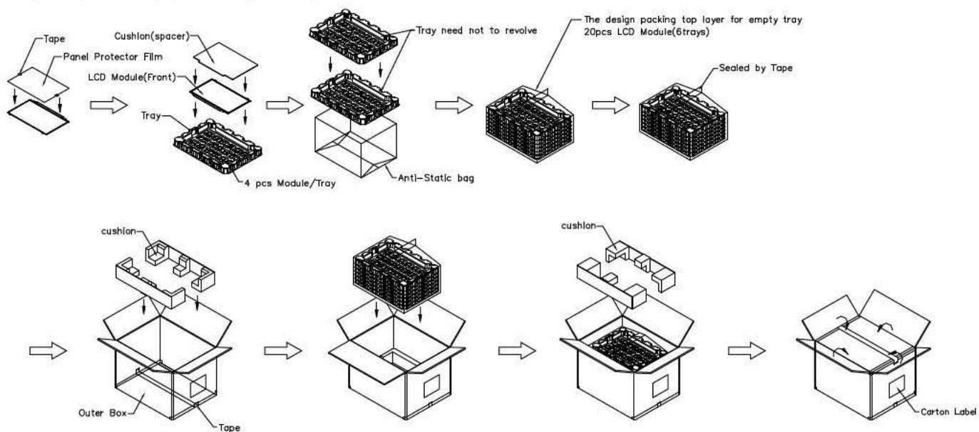
Figure. 7-2 Packing method
