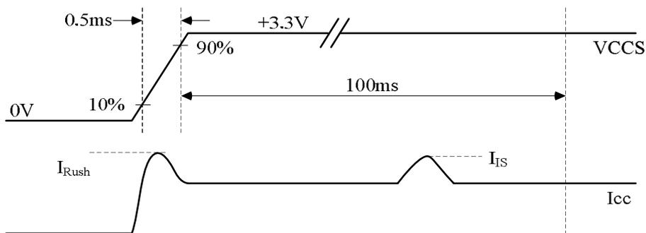
Note (3) The specified power supply current is under the conditions at  $V_{CCS} = 3.3\text{ V}$ ,  $T_a = 25 \pm 2\text{ }^\circ\text{C}$ , DC Current and  $f_v = 60\text{ Hz}$ , whereas a power dissipation check pattern below is displayed.
