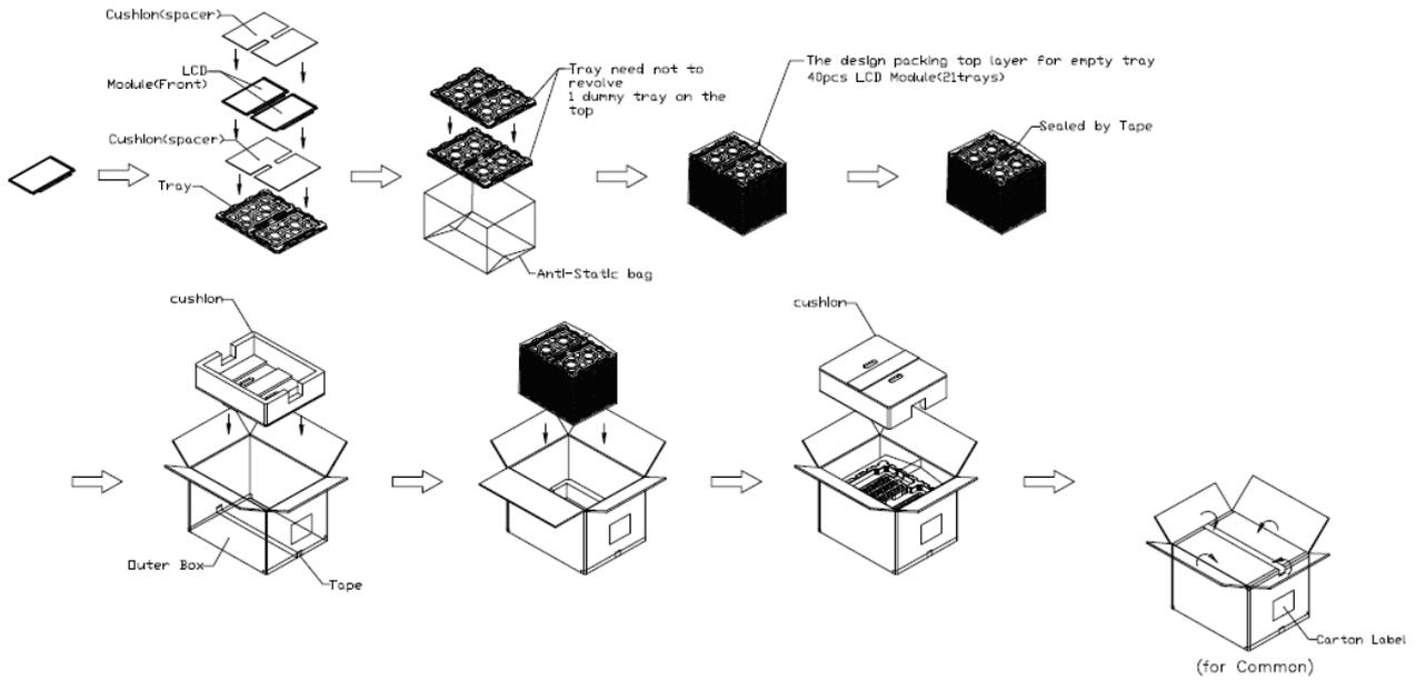
Figure. 7-2 Packing method
