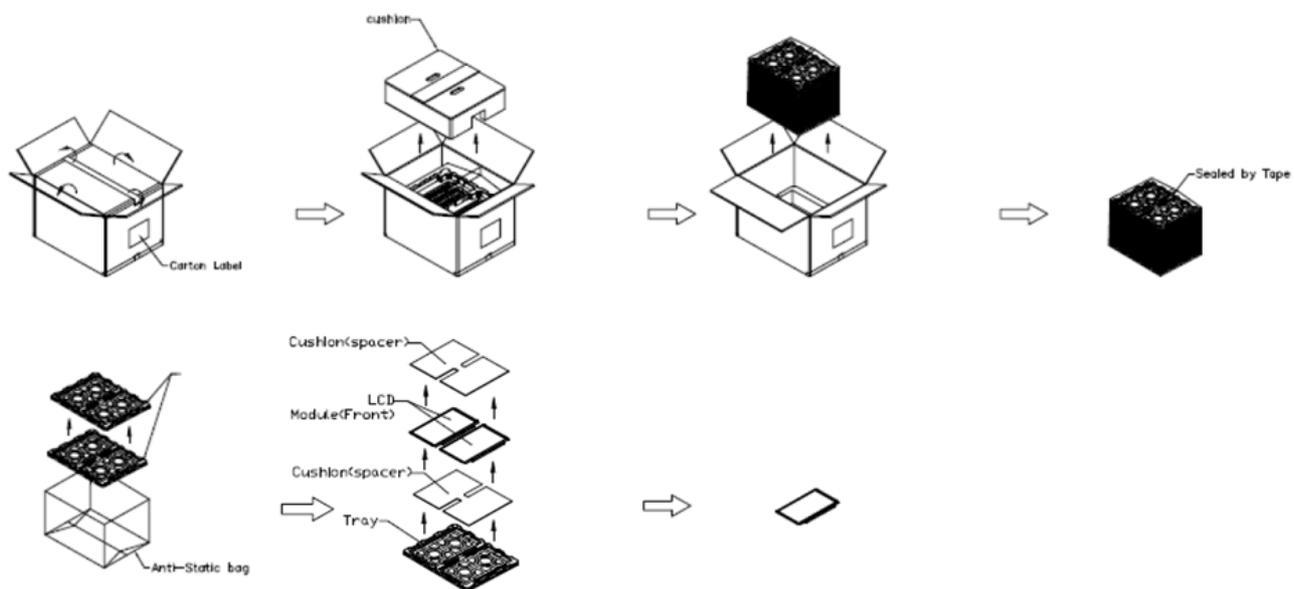
**Figure. 7-3 Un-Packing method**
