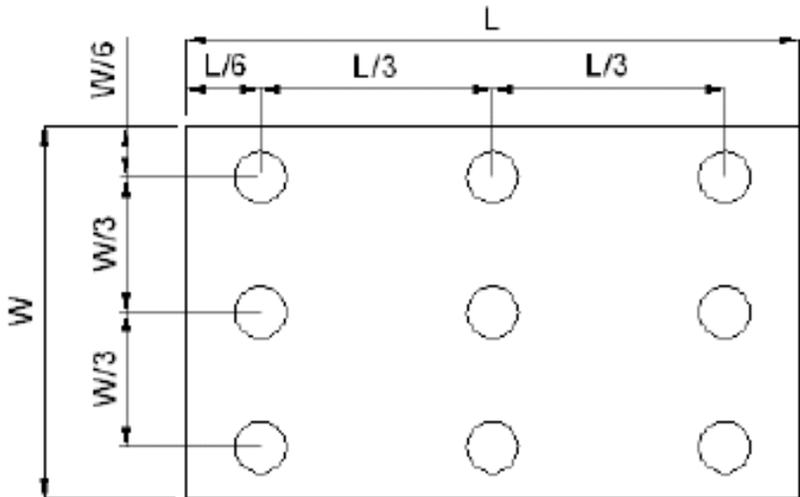
Center Luminance of white is defined as luminance values of center 5 points across the LCD surface. Luminance shall be measured with all pixels in the view field set first to white. This measurement shall be taken at the locations shown in FIGURE 2 for a total of the measurements per display.
