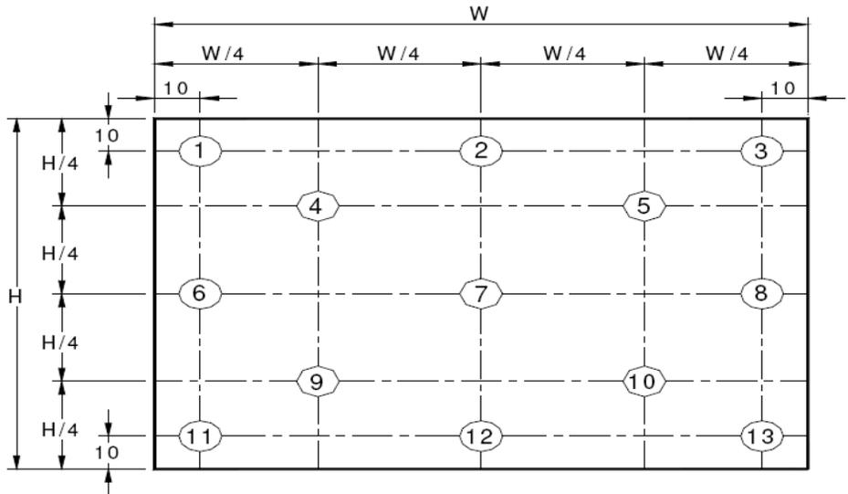
The White luminance uniformity on LCD surface is then expressed as :  $\Delta Y_{13} = \text{Minimum Luminance of 13 points} / \text{Maximum Luminance of 13 points}$  (see FIGURE 3).
